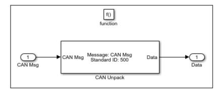
The reason to place the CAN Unpack inside a Function-Call Subsystem is so that it can capture all possible messages.
