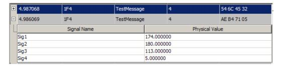
The tool displays the signal name as defined in the attached database and the signal's physical value.
