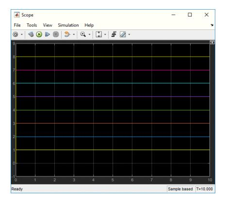
In the graph, the horizontal axis represents the simulation time in seconds and the vertical axis represents the received data value. You configured the model to pack and transmit an array of constant values, [1  $\,$ 2  $\,$ 3  $\,$ 4  $\,$ 5  $\,$ 6  $\,$ 7  $\,$ 8], every 0.01 seconds of simulation time. These values are received and unpacked. The output in the Scope window represents the received data values.
